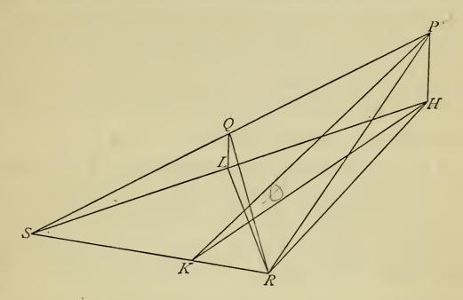
pendicular to RS, and PH and QL perpendicular to the plane RHS. Then RHL is equal to the projection of PQR on the given plane.
